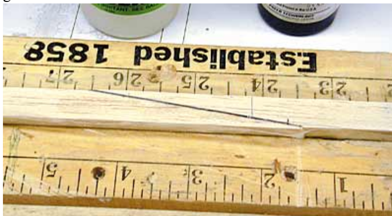
7 The finished splice.
